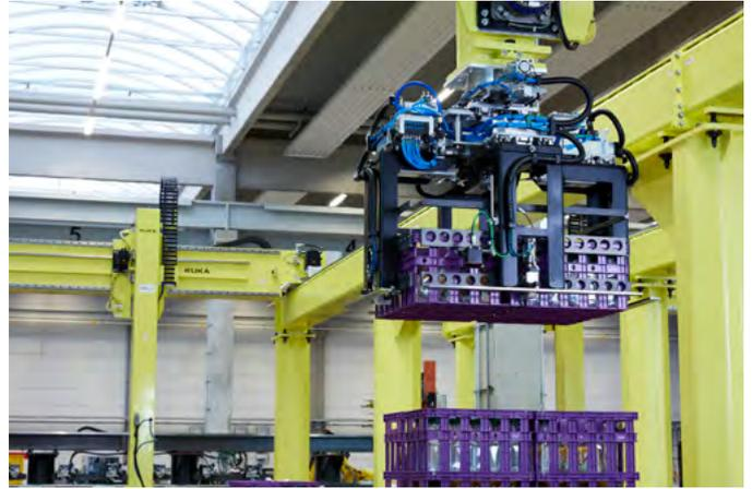
The KUKA robot is able to pick up an entire layer of drink cartons using its mechanical gripper.
