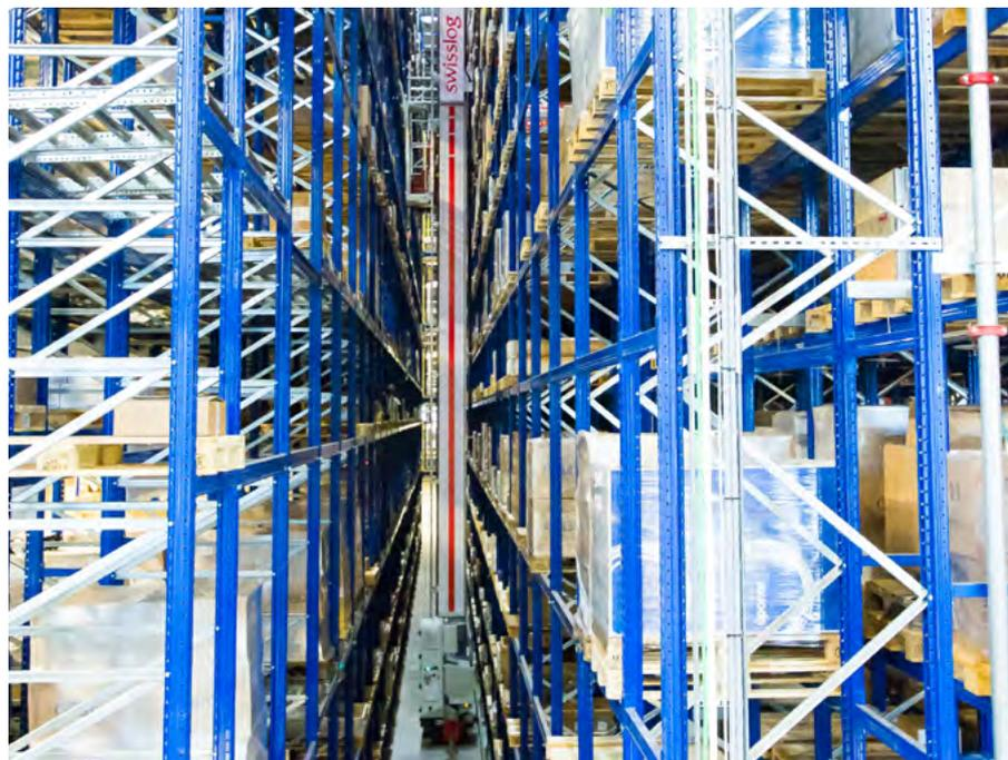
The Vectura automated storage and retrieval stacker crane from Swisslog provides reliable handling of pallets in the Almarai high-bay warehouse.
