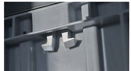
The robot's gripper plate hooks securely into the respective storage bin for transport.
