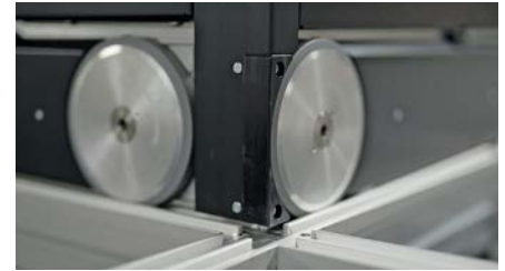
Pairs of wheels arranged at right angles give the robots complete freedom of movement around the grid.
