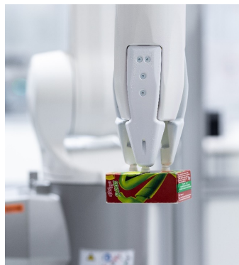
Three fingers for light or instable items
