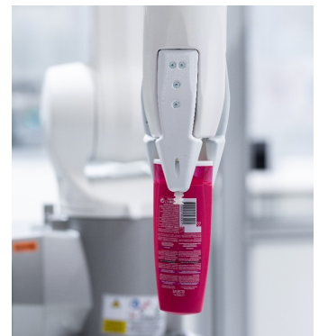
Central suction and hold for bottle shaped products
