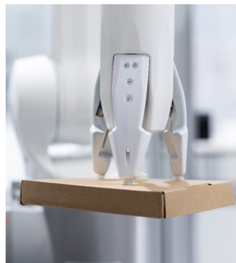
Central unit plus three fingers for large items
