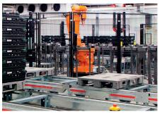
ProMove is an efficient and fully-automated transportation system for palletized goods which can move pallets horizontally and vertically in any warehouse Swisslog's ProMove pallet conveyor system is based on proven, standard elements and can be configured to accommodate demanding requirements from a variety of customers. ProMove connects your warehouse — with its modular design and a standard interface — to other sub-systems, allowing fast and efficient warehouse processes.
