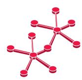
A distributed system offers unlimited scalability. To grow the system, you add more nodes, which only have to communicate with a limited number of related nodes to connect to the entire system.
