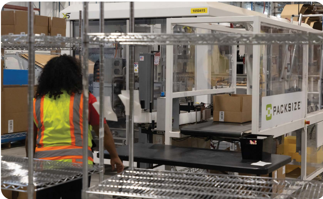
Cartons are created on-demand in the automated packaging system.
