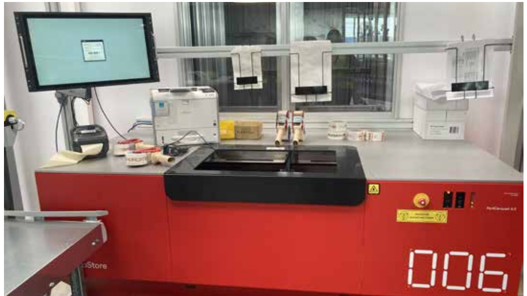
A pick station equipped with screen for SynQ.
