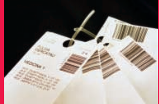
The unit-doses are assembled on the PickRing. A bar-code system ensures the identification of the bags.
