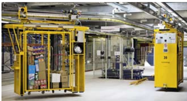
CaddyPick is based on a computer-controlled electric monorail system, enabling efficient picking of transport units for individual outlets.
