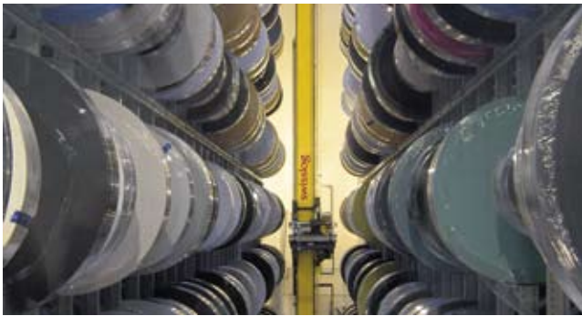
The modular Vectura stacker cranes are applicable in a large number of industries; in this case, at a warehouse for highly sensitive plastic film.
