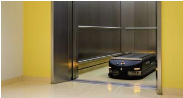
The laser-guided Automated Guided Vehicles (AGV) navigate independently throughout a building, including different floors.
