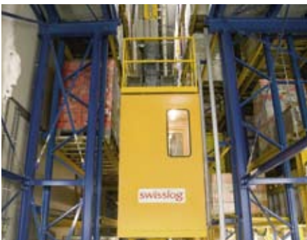
View of control box of stacker crane in a high-bay warehouse (left)
