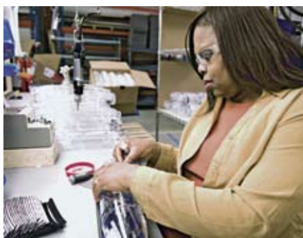
Assembly of pneumatic tube carrier (left)
