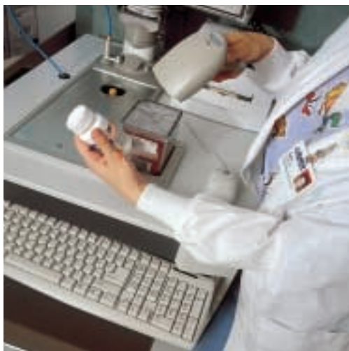
An employee of the hospital pharmacy at Erlanger scans the barcode of a drug and thus feeds the specific information of the preparation in the drug management system.
