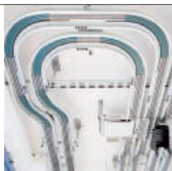
Fast and safe transport on overhead mounted track with curves and transfer switch
