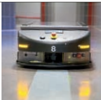
Modern, redundant security technology allows a safe material transport with automated guided vehicles (AGVs)
