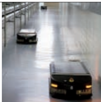
Free navigating, laser-guided TransCar LTC 2 in hospital supply tunnel
