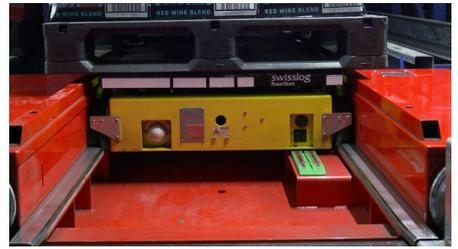
Together, the Aisle Carrier and Row Carrier pair deliver and retrieves pallet loads from the rack.
