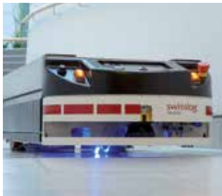
TRANSCAR Automated guided vehicle for voluminous goods transport.
