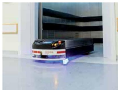
On the way to its destination, the system automatically selects an appropriate elevator and activates it through wireless communication. Doors along the route are automatically opened.
