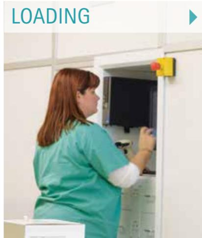
A technician logs into the BoxPicker operator station and selects the Load option
